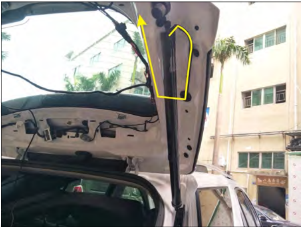
5. Right Hall line lead routing.
