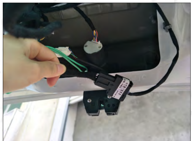
13. At the rear door lock position, unplug the original car socket and insert our three-way socket. And the other end three-way plug back the lock.
