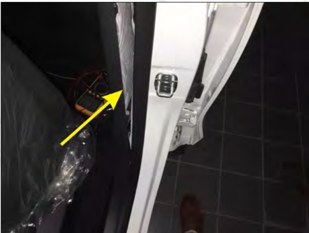
11. Remove the trim panel at the main driving seat belt B-pillar and find the central control.
