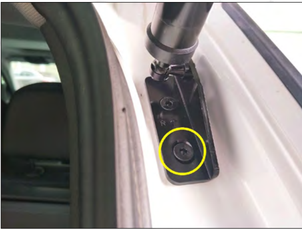
3. Remove the original right lower bracket. Install our right lower bracket and fix it with our screws.
