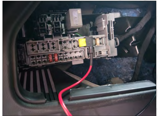
6. Remove the trim panel on the left side of the tailgate and find the power supply.
