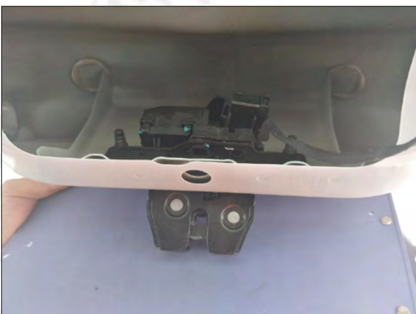
13. At the rear door lock position, unplug the original car socket and insert our three-way socket. And the other end three-way plug back the lock.
